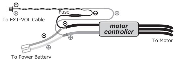
The connection is affixed to the ESC on the wires that are connected to the battery by soldering them and then protecting them with heat shrink.
